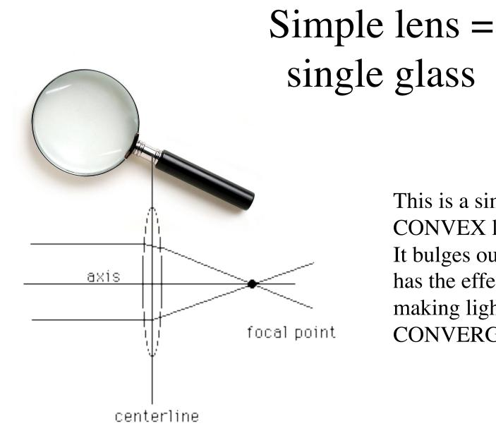
This is a simple **CONVEX** lens It bulges out, and has the effect of making light **CONVERGE**
