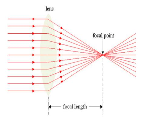
A key aspect of any lens is its FOCAL LENGTH, the distance between its **OPTICAL CENTER** and the FOCAL POINT where rays of light from infinity converge.
