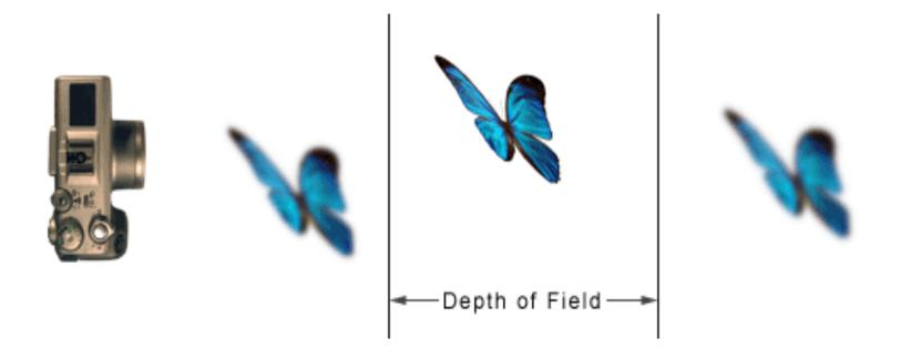
Telephoto lenses have a shallow or narrow depth of field, While wide-angle lenses have a broad depth of field.
