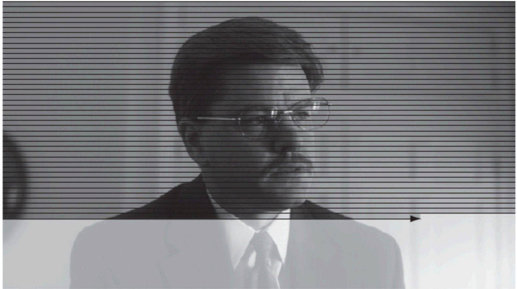
■ Figure 9-4 Progressive scanning draws a full frame of video, from top to bottom, with each pass.
