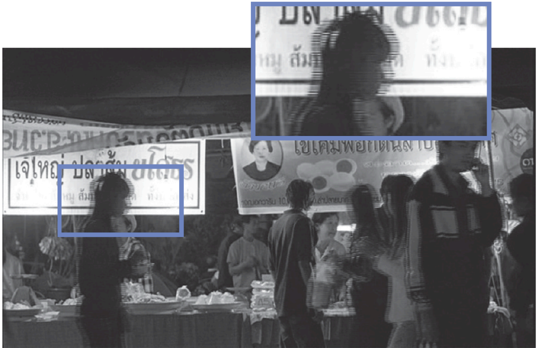
■ Figure 9-5 When interlaced video is shown on progressing displays, a “combing” artifact occurs at the edges of moving objects caused by the displaced scan lines (notice that the stationary objects do not show any combing).
